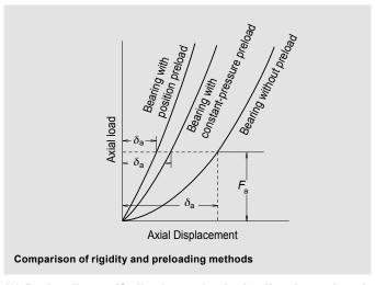
$$F_{\text{a min}} = \frac{C_{0\text{a}}}{100} \cdot \left(\frac{n}{N_{\text{max}}}\right)^2$$
