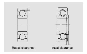
Internal clearance has a major impact on the operating performance of bearings. It affects factors such as their service life, vibration, noise level and heat generation.
