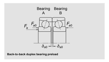
Bearing rigidity – i.e. the relationship between load and axial displacement – with a given axial load F<sub>a</sub> imposed on a duplex set.
