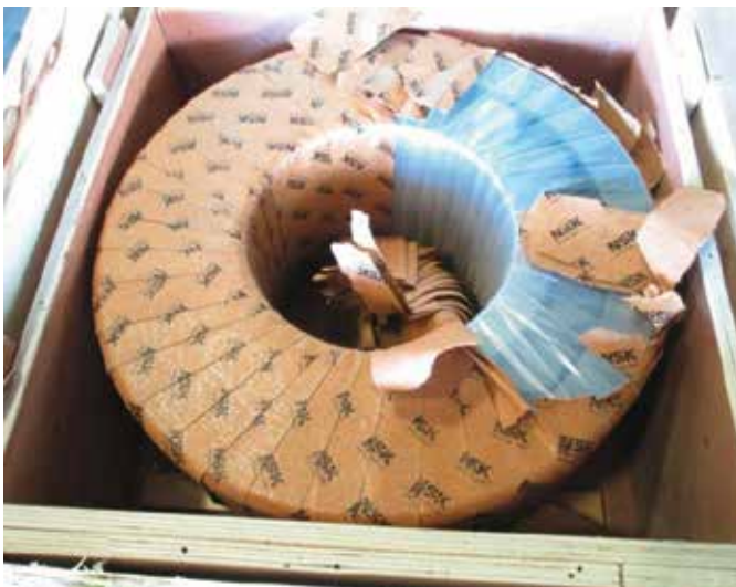
Both images are counterfeit. Incorrect wrapping and no markings on bearings.
