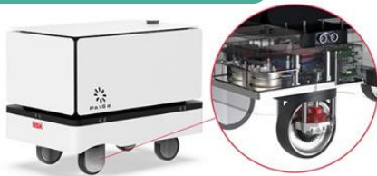
Drive units enabling smooth omnidirectional movement, such as the active caster PalGo.
