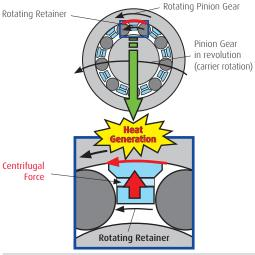
Higher-speed design of planetary  $\rightarrow$  Generation of seizure and abnormal wear
