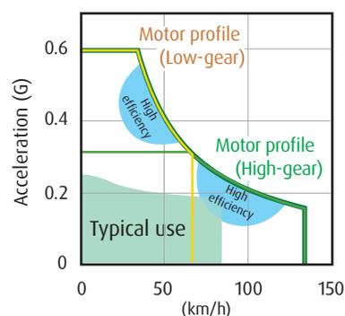
**Max torque: 850Nm (Low-gear)
