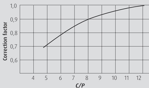
Relationship between the correction factor and the load ratio
