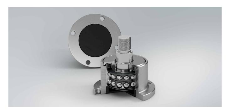
NSK's Flanged Bearing Unit (4,5,6 holes) with integrated shaft sealing and a angular contact ball bearing with 40 ° contact angle. Specially designed to be interchangeable, maintenance free, increasing the machinery's availability and reliability in extreme conditions. For applications that include cover-crop, front-packer, seeding, row cleaning, mowing and finger-weeding.
