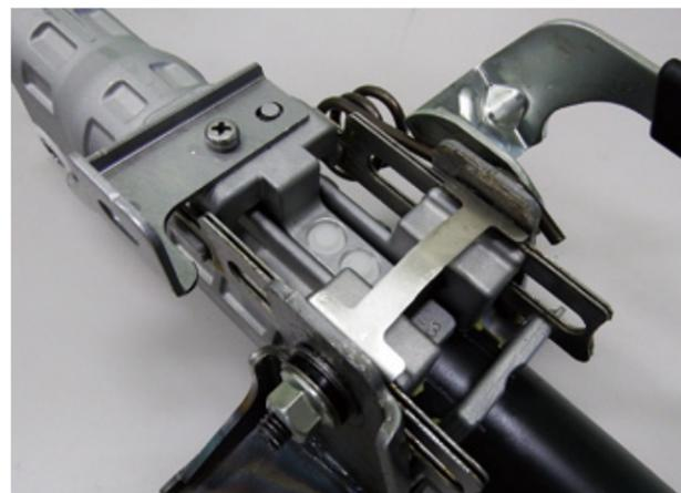
Photo 2 New breakaway mechanism portion
