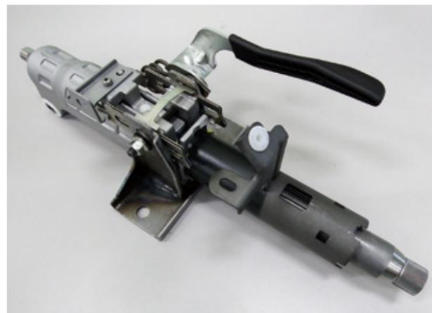
Photo 1 Steering column with the newly developed product
