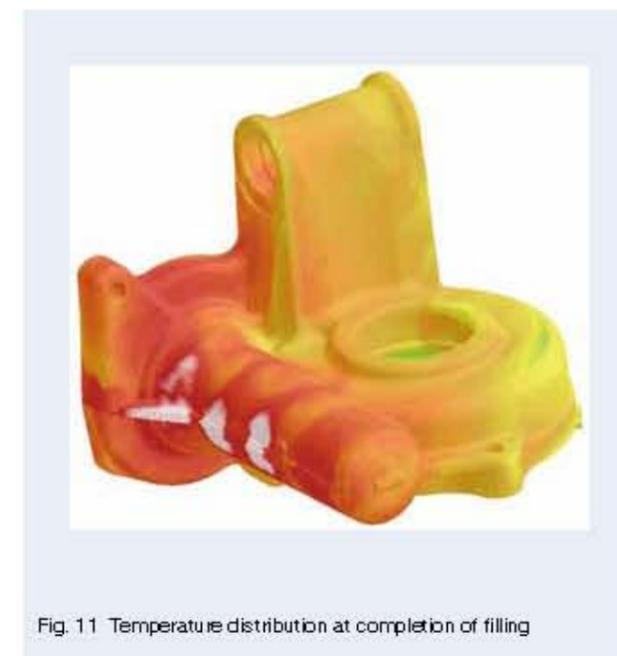
Fig. 11 Temperature distribution at completion of filling
