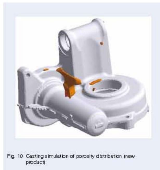
Fig. 10 Casting simulation of porosity distribution (new product)
